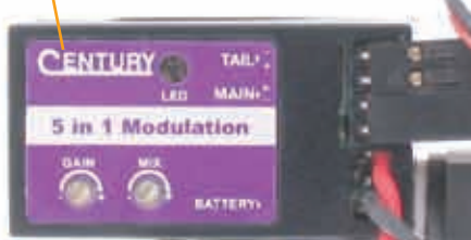
(For advanced users: Gain modifies gyro sensitivity. Mix modifies tail motor power)
