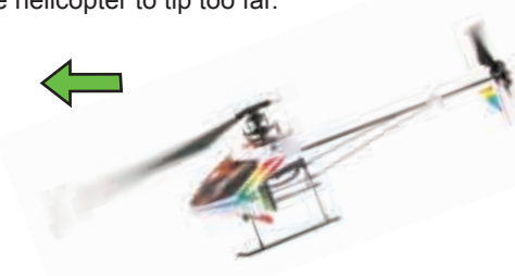
Helicopter tilts/drifts forward by adding upward Elevator input.
