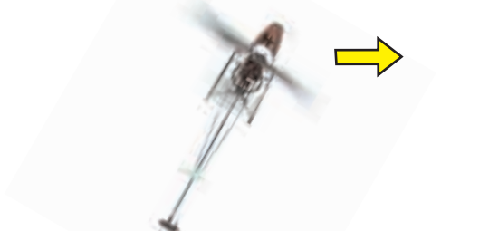
Helicopter nose moves right by increasing the tail motor speed.
