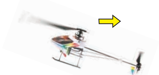
Helicopter tilts/drifts reverse by adding downward Elevator input.
