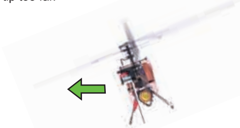
Helicopter tilts/drifts left by adding left Aileron input.
