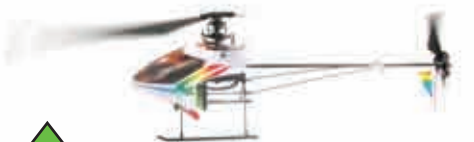
Adding throttle moves the helicopter higher in the air by increasing speed to the motors.
