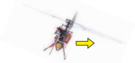
Helicopter tilts/drifts right by adding right Aileron input.
