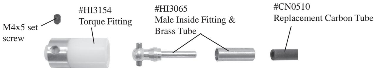
3. Having completed one end, measure and cut the tube to fit your helicopter. Cut the tube by wrapping with masking tape and use a moto-tool with a cutoff wheel.
